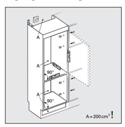
Before installing the appliance the housing unit must be carefully aligned using a spirit level. The unit corners must be at right angles, as otherwise the furniture door will not align correctly with the 4 corners of the appliance.
